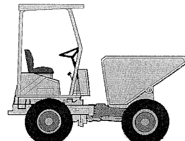
A detailed line drawing of a minidumper truck, shown from a side profile. It features a high cab with a steering wheel, a large front-mounted engine compartment, and a large, open-topped dump bed at the rear. The truck has two large, heavy-duty tires. |
